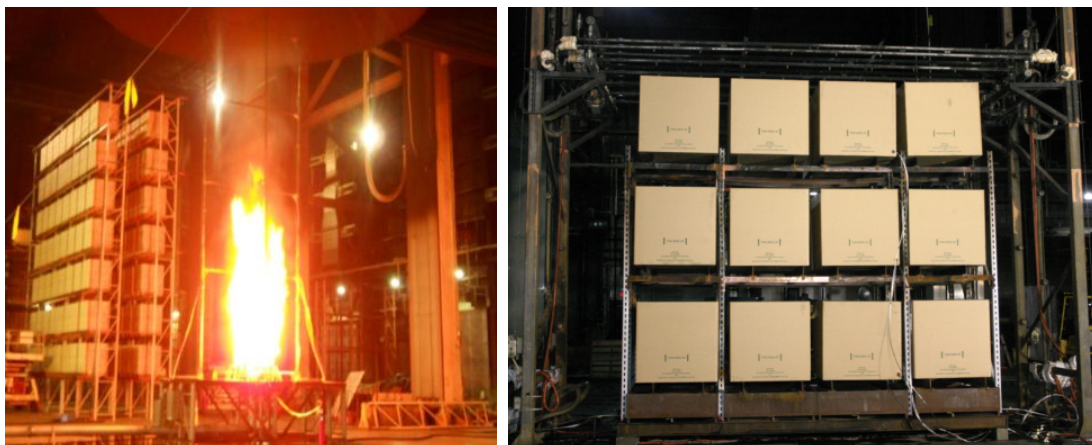
Figure 12 ADD and WAA tests under 20-MW calorimeter.
