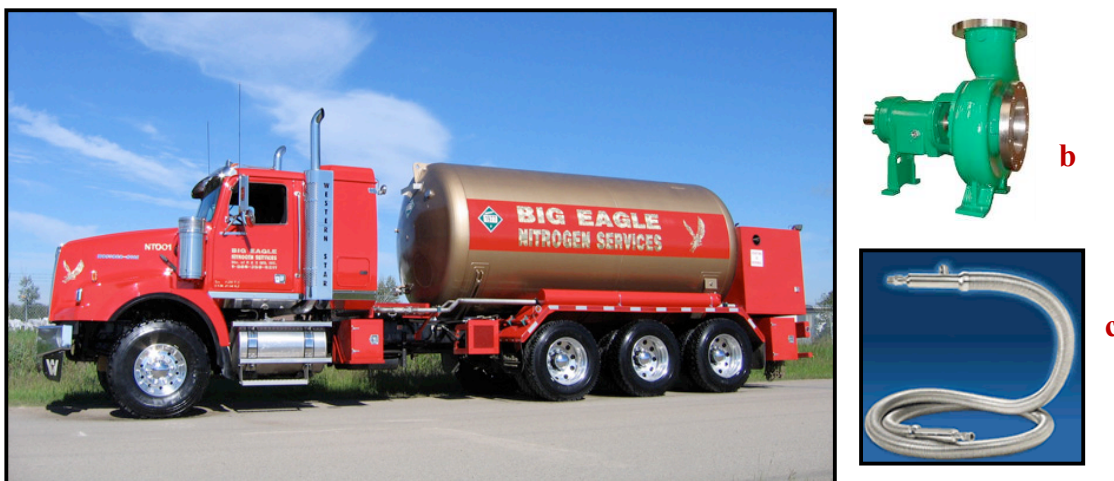
Figure 1. Photographs of (a) a commercial liquid nitrogen truck, (b) cryogenic pump and (c) hose.
