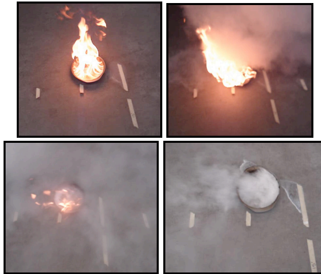
Figure 3. Photographs of fire extinction of a small alcohol-fueled fire, set at a distance of 5 meters away from the LN 2 nozzle. (i) Time: 0s, LN 2 valve is opened. (ii) Time: 7s, small quantities of liquid LN 2 reach the fire. (iii) Time: 36s, increasing quantities of liquid LN 2 reach the fire. (iv) Time: 90s, the fire is extinguished.
