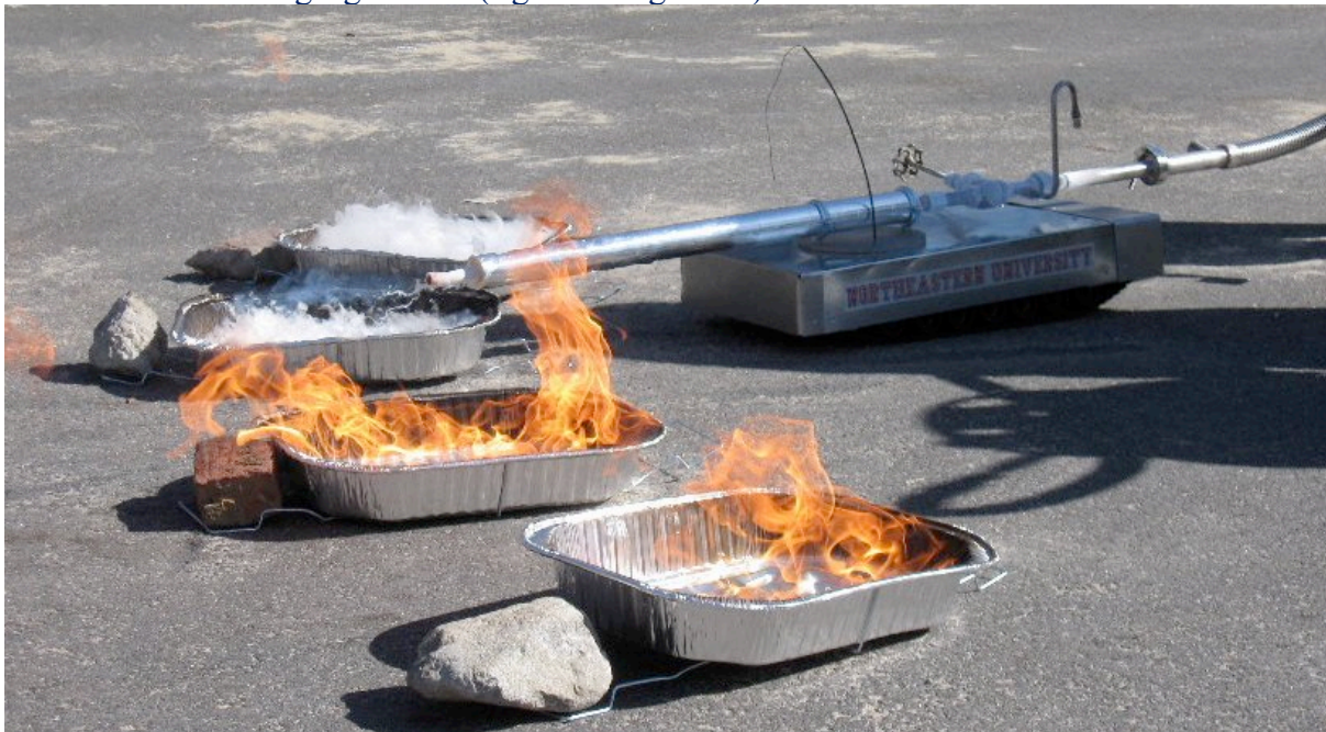
Figure 5. Fires of iso-propanol burning in four aluminum pans in a staggered arrangement were extinguished by a remotely-controlled vehicle, which distributed LN 2 to the fires in a zigzag motion (right-left-right-left) as it moved forward.
