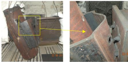
Figure 7. Typical failure of reverse-channel connection to CFT column.
