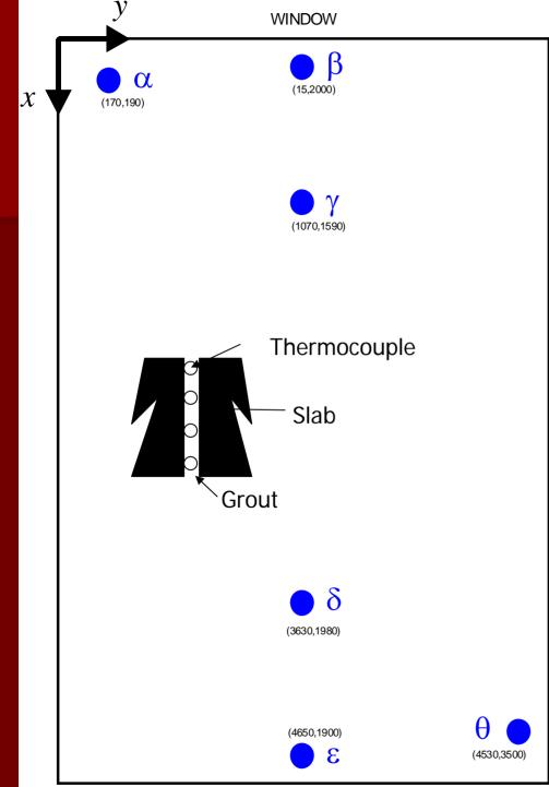
Thermocouple locations6 stations in plan4 t-cs at each stationHoles grout-filled
