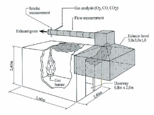
Figure 2. The ISO 9705 Room Corner test
